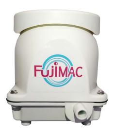
A FujiMAC 80, pictured, delivers 80 litres per minute (1055 gallons per hour) of air to the treatment process using only 47W of electricity, at 36dBA, 10dBA quieter than alternatives and saves more than £50 on electricity per year on a typical 6-population installation.
